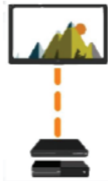
In-Wall Cable Chase 110v Outlet at 5' Off Floor for TV
